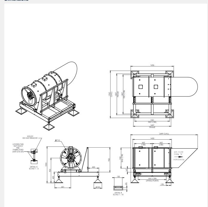
The above drawing dimensions illustrate a typical TITAN7-M5-F2 dual fan set.
