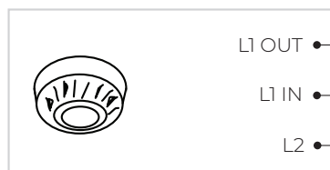
SSR3 - SMOKE SENSOR
