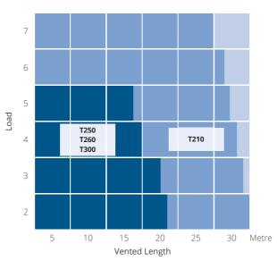
LOAD = No. of chain openers + No. of bends in conduit
